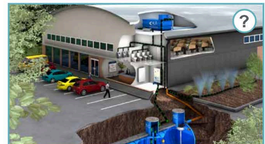
Plate 89 - Rainwater harvesting. Source: Stormwater Ltd.
