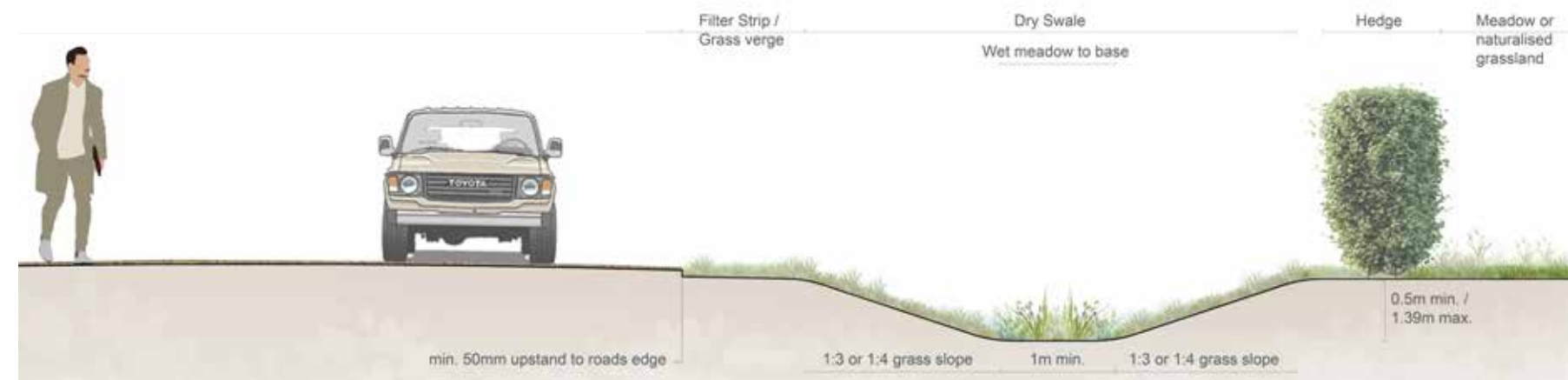
Plate 64 - Typical cross section through drainage swale
